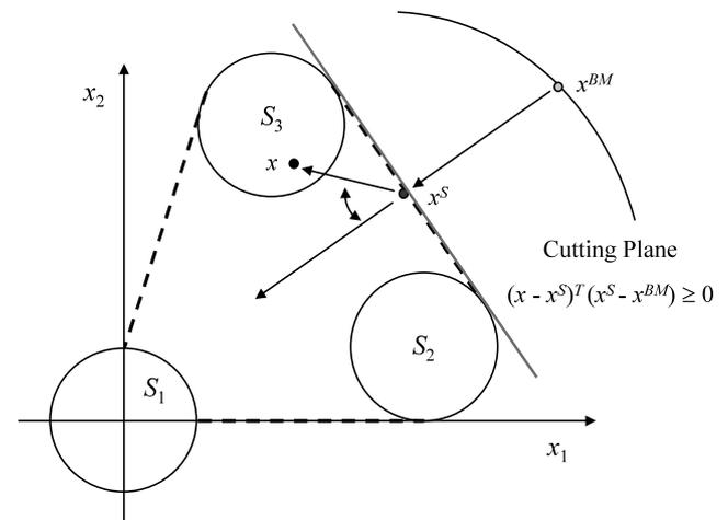
Fig. 13. Cutting plane generated by separation problem.
